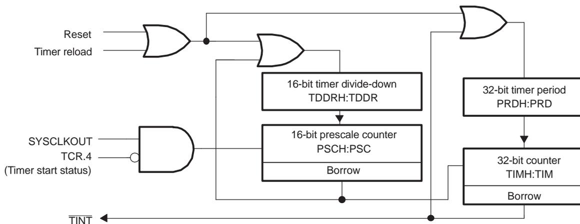
Figure 37. CPU-Timer Interrupts Signals and Output Signal
